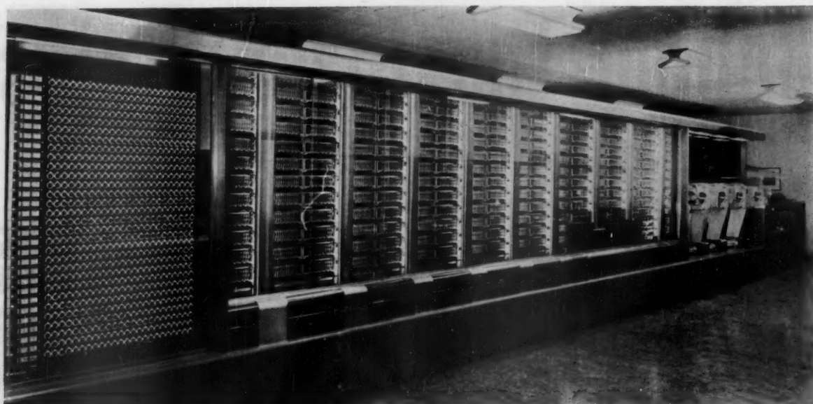
All computing and processing of information in the Harvard Mark I was performed by means of high-speed relays. This is what the calculator looks like today, after some modifications have been made.
